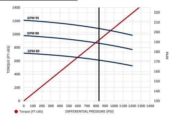
Stator and Rotor sizes are subject to change at the discretion of Adtech. Power section specifications may vary due to environmental conditions. Operation of power section above the maximum recommended differential pressure will result in a decrease of stator life and performance.
